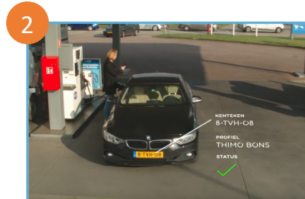
2 License plate is recognized and recorded in the system
